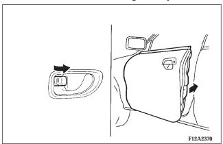
To lock the door, set the inside lock knob to the locked position, and close the door.
